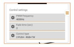
On the *Control Settings screen,* you can configure the different parameters for the driver's operation mode.
