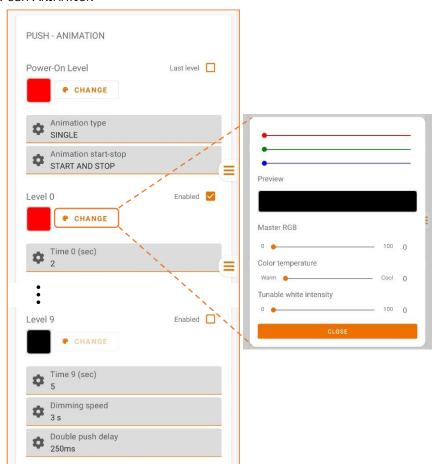
**Power-On Level: Sets** the RGB and white light levels to which the output is brought as soon as the device is powered. The RGB and intensity parameters can be set via the "Change" submenu.
