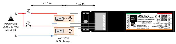
Figure 8: Local Command connection diagram for Long Distances
