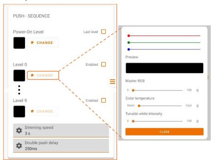
**Power-On Level: Sets** the RGB and white light levels to which the output is brought as soon as the device is powered. The RGB and intensity parameters can be set via the "Change" submenu.
