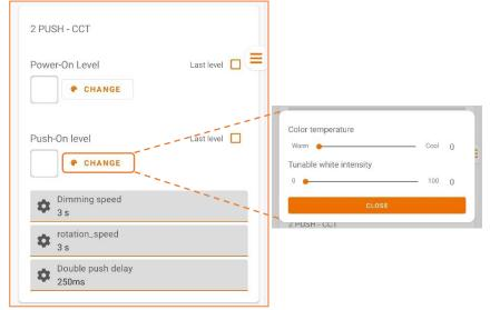
**Power-On Level: Sets** the white light levels to which the output is brought as soon as the device is powered. The intensity and colour temperature parameters can be set using the "Change" submenu.
