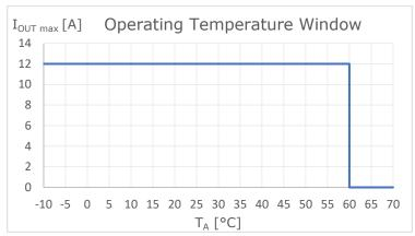
Figure 11: Operating Temperature Window
