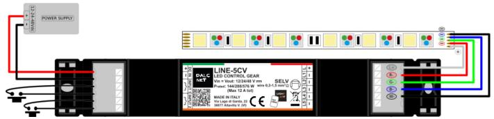
Figure 5: Connection diagram for RGBW LED load
