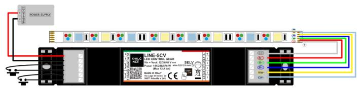
Figure 6: Connection diagram for RGB+TW LED load
