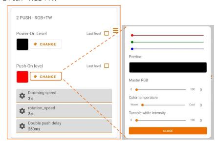
**Power-On Level: Sets** the RGB and white light levels to which the output is brought as soon as the device is powered. The RGB and intensity parameters can be set via the "Change" submenu.
