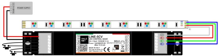
Figure 4: Connection diagram for RGB load
