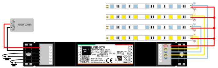
Figure 3: Connection diagram for Tunable White LED loads
